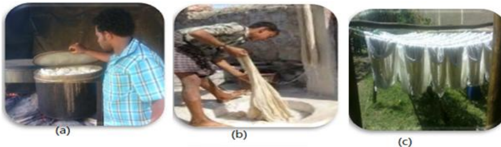
Fig 2. Warp yarn sizing - (a) squeezing (b) drying (c) in traditional weavers
