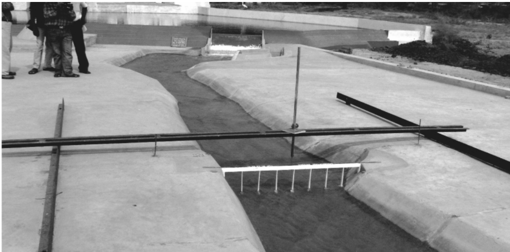
Figure 1: Physical Model River reach from Ukai dam to D/S of Hindustan Bridge (Suthar, 2011)
